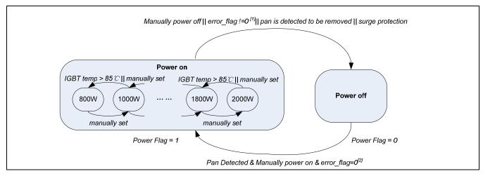
Figure 3-1 State Transition Diagram
